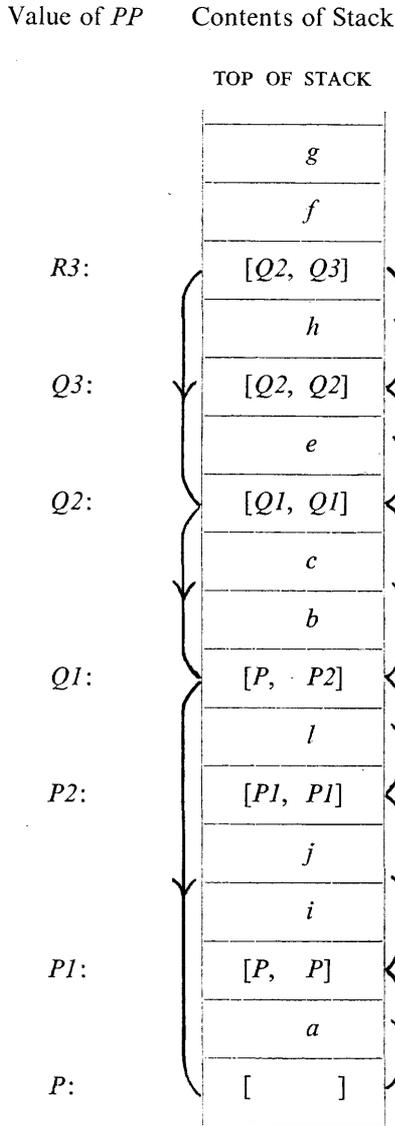
FIG. 1(b). Stylised Representation of contents of stack, as at label  $L$  in procedure  $R3$ .
