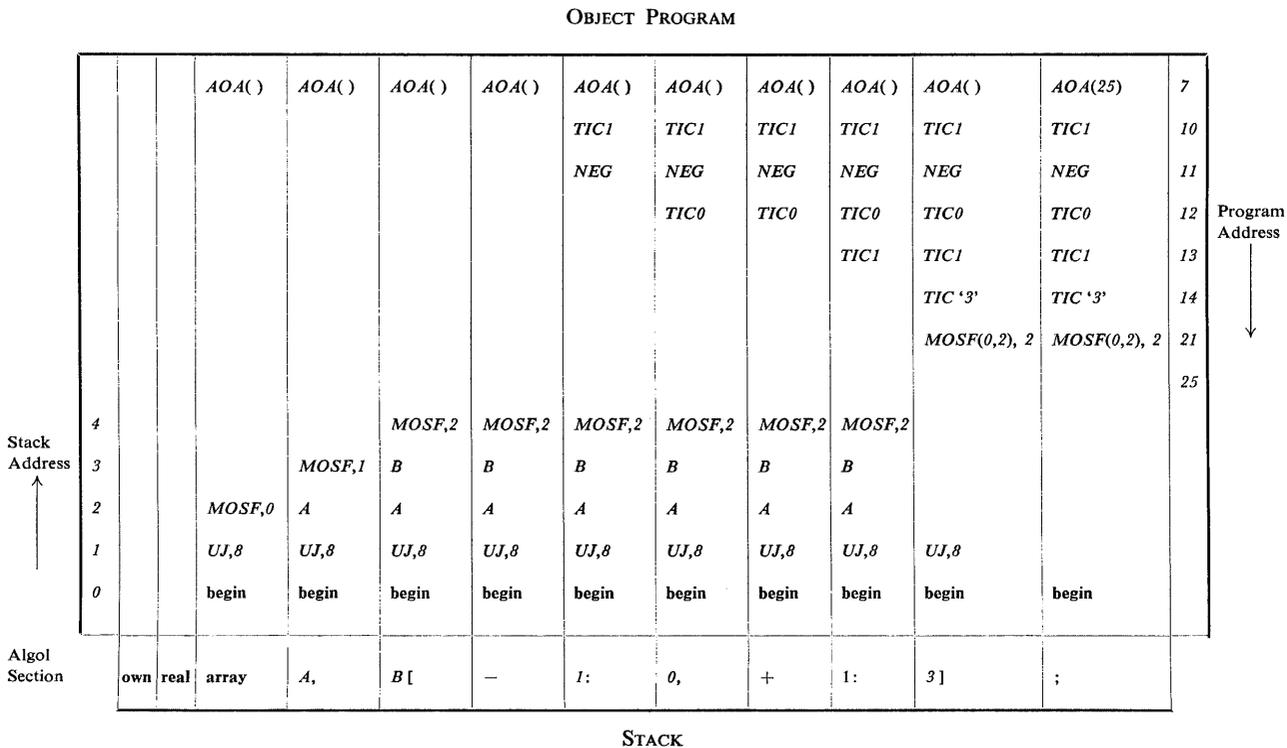
FIG. 11. Representation of Object Program and Stack at each stage during the translation of an own array declaration.
