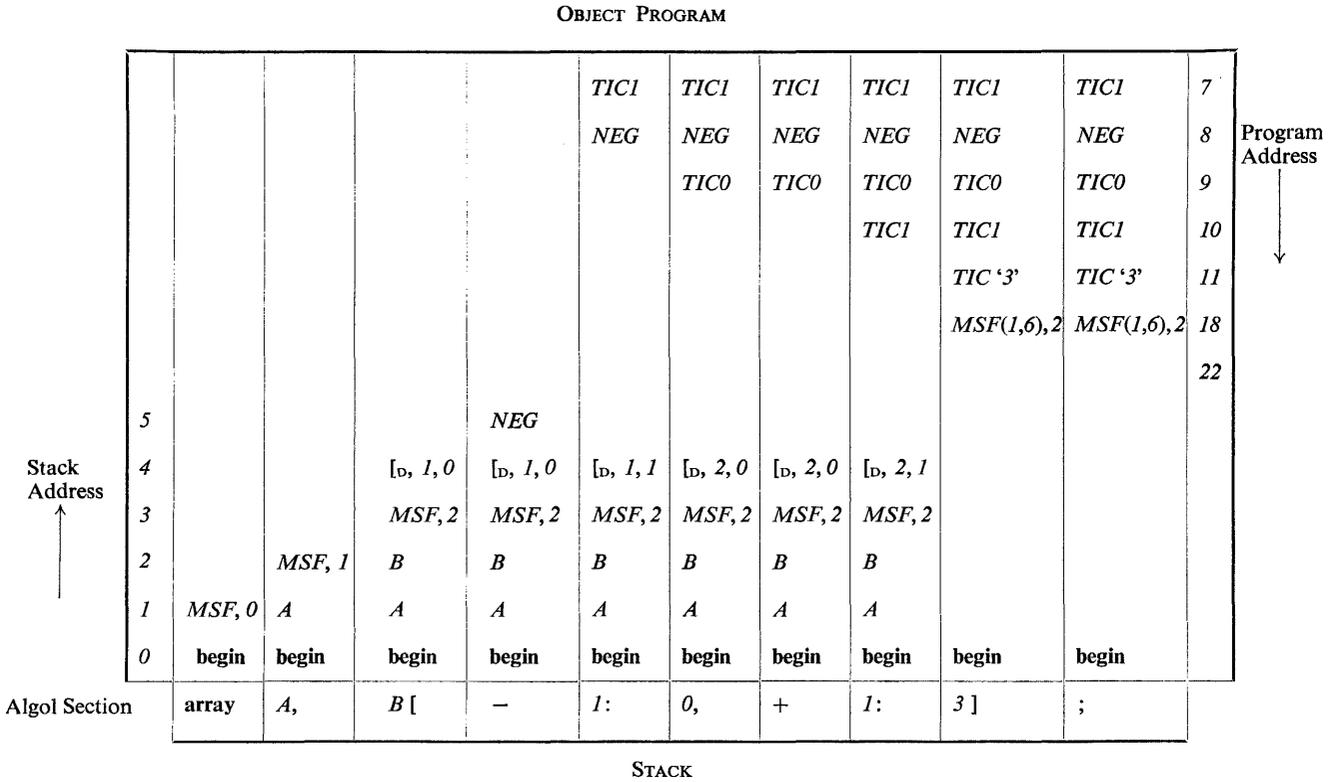
FIG. 10. Representation of Object Program and Stack at each stage during the translation of an array declaration.
