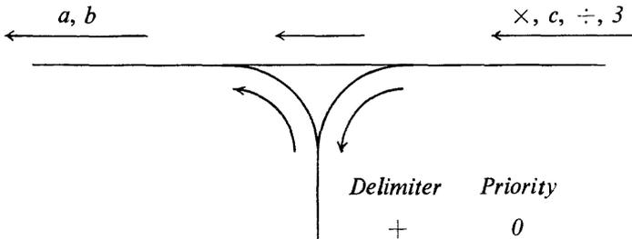
The delimiter 'x' with its priority of one cannot cause the '+' to be unstacked before it, too, is stacked. The identifier  $c$  transfers straight to the output and the picture is as follows
