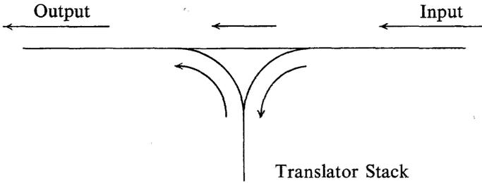
The shunting yard has the form of a 'T' junction with the translator stack as the branch line to perform the 'shunting' or re-ordering. Identifiers or constants pass straight from input to output but in general the delimiters reach the output via the translator stack. Before the delimiters are shunted into the translator stack any delimiters at the top of the stack which have a priority equal to or greater than that of the current delimiter, are allowed to pass to the output.
