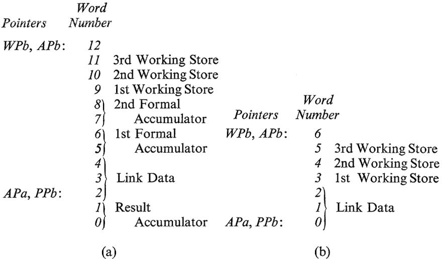
FIG. 3. Stack Reservations on Entries to Procedures and Blocks. (a) Procedure with two formal parameters, three working stores. (b) Block with three working stores.
