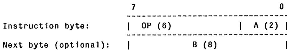
Most instructions read from or write to an "effective address", and possibly also push or pop 32-bit words on the stack. When the OP field indicates that an effective address is to be read from, it is computed from the A field and (sometimes) from the subsequent byte B as follows:
