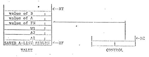
Now, we link to the function application routine. This routine moves up the stack pointers. That is, XF is saved in the control stack, the address of the code representing the function is picked up (top of control stack points to word containing it), the return address and association list are saved in this word, XF is changed to the new base, end the function is jumped to. Now the stacks look like:
