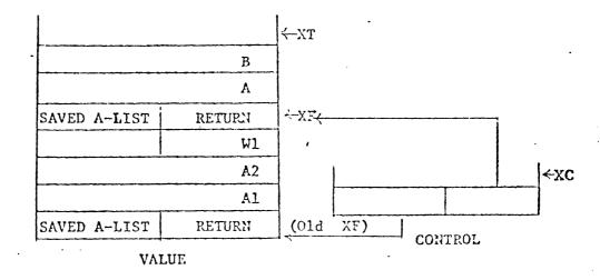
Now the stacks have been pushed up and we can execute the code for the function that was just entered. When we have the result computed, we leave it in a specified register and leap to the exit routine. The exit routine simply undoes everything and leaves the stacks just like they were before with the result pushed into the top of the value stack (it is also possible to simply leave it in its register without pushing it into the value stack).
