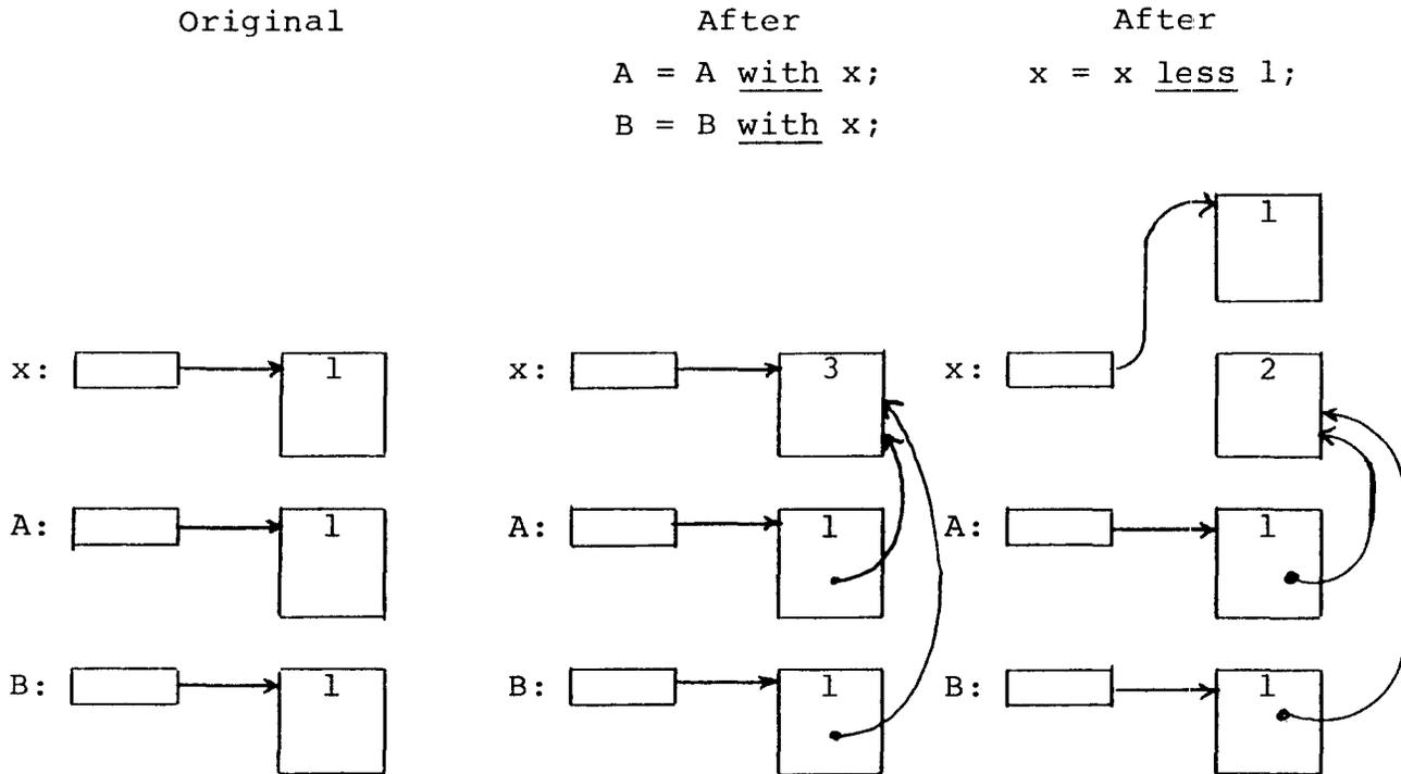
point to data structures in the storage heap when their values won't fit in the "root word". The numbers in the data structures of the above figure are the reference counts.
