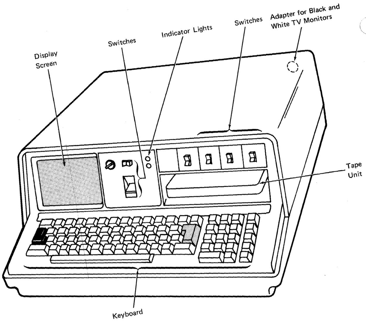
Figure 1. IBM 5100 Portable Computer
