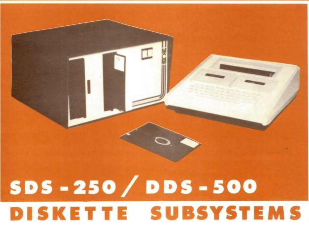
The MCM DISKETTE SYSTEM provides the user with totally random on-line storage. Access time for any random files are typically one second, under control of the MCM Virtual Memory System. In order to meet the demands of both large and small applications, MCM offers two models - the SDS-250 Single Diskette and the DDS-500 Dual Diskette Systems. With the exception of the additional disk in the DDS-500, both systems are identical.
