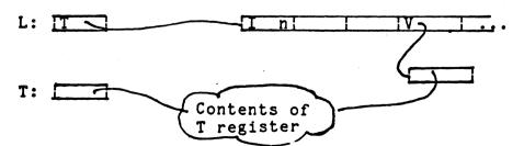
If the source and destination are actually both the same variable then the S instruction performs no operation. (If the normal mechanisms were to apply a link would be set up in the target word to itself! This is extremely dangerous and could
